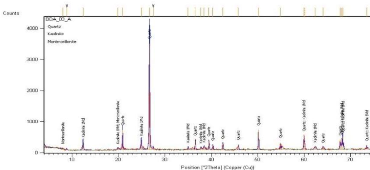
**Figure 7:** XRD result of sample BDA/03/A
