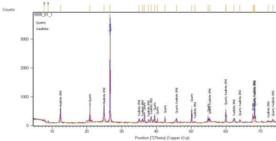
Figure 10: XRD result of sample BBB/01/A
