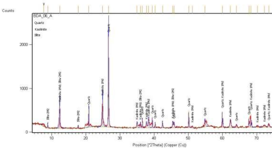
Figure 9: XRD result of sample BDA/06/A
